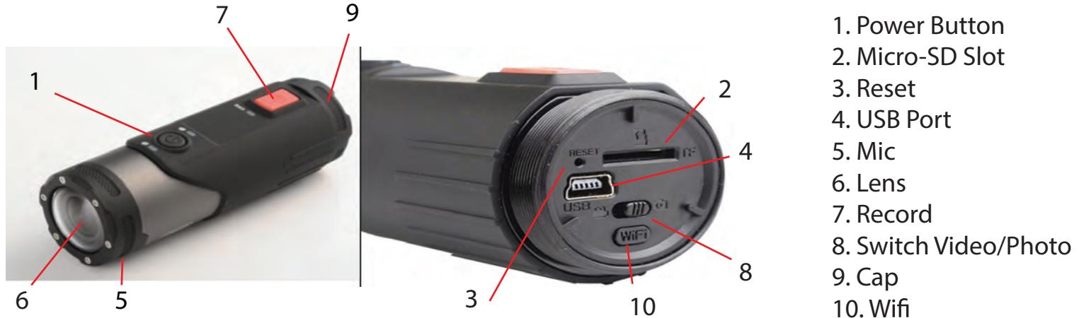
To access the sd card slot / USB / Wifi unscrew the cap (9) at the bottom of the camera)
